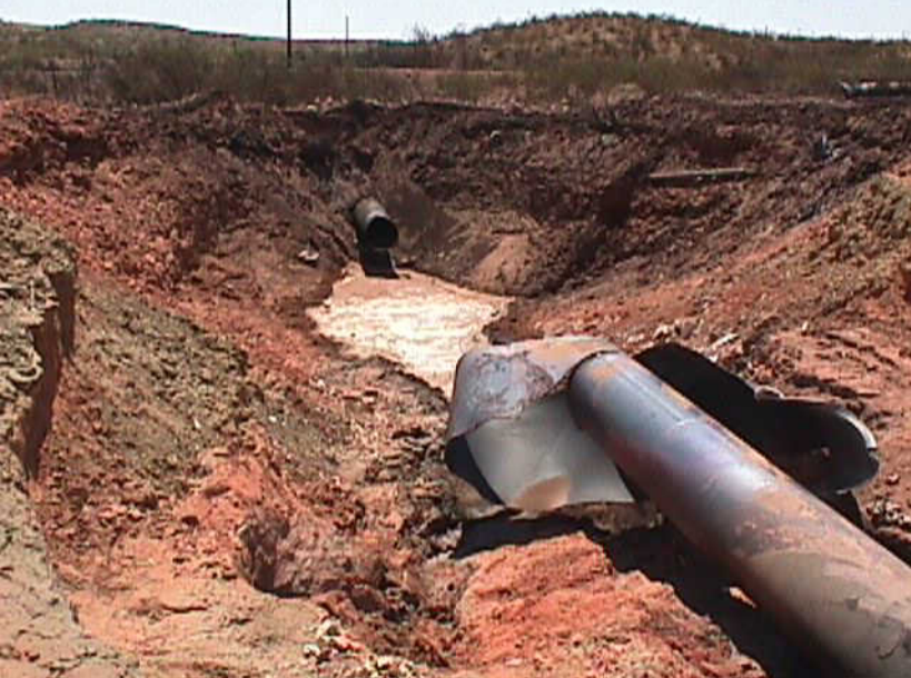
Photo of ruptured El Paso Natural Gas Company pipeline in crater at Carlsbad, New Mexico
