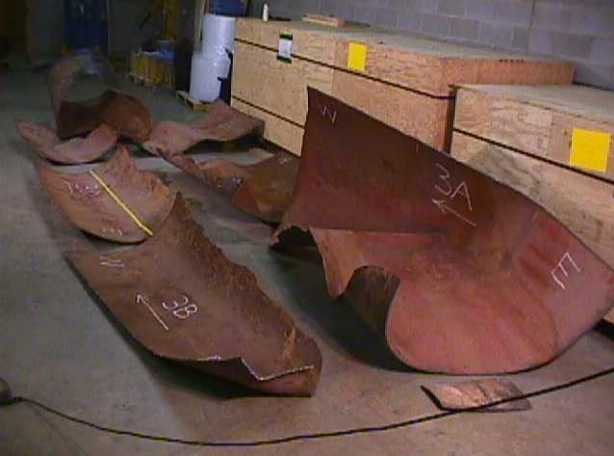
Photo #1 - pieces of ruptured pipe in NSTB lab
